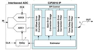
**Test case**: a 20-tone, wideband signal is used to test a simulated 14-bit/3Gsps/64dB SNR/3GHz BW, time-interleaved ADC with 0.25dB, 5ps and 200MHz gain, time skew and bandwidth errors respectively. Interleaving spurs limit the SFDR to -50dBFS before calibration. CiP2016 IP cancelled effectively these spurs down to ADC noise floor.
